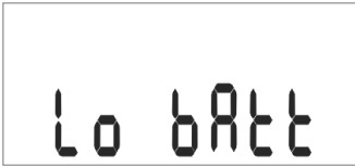
Figure 5: LCD showing LOW Battery indication
